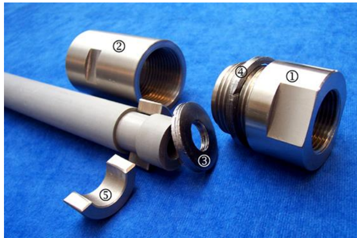
Adapter parts with Syalon protection tube, text above describes the numbers
